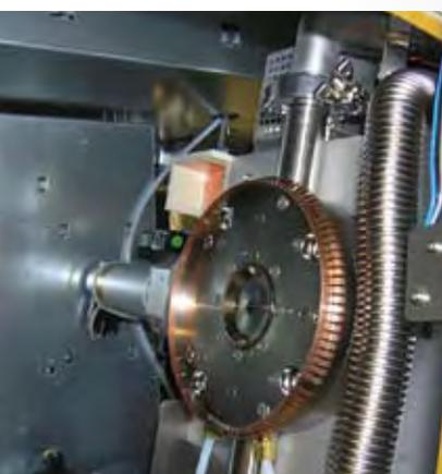
*With an open sample chamber, visual examination of the cones can be easily conducted. If necessary, the entire component block can be brought, with a mouse click, into the service position so that cones or extractor lens can be serviced.*
