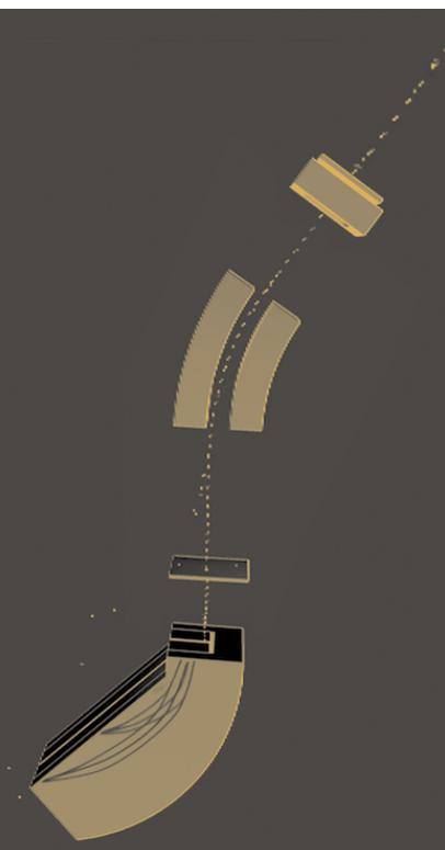
*Simultaneous measurement of the entire spectrum is enabled by the combination of double focusing sector field mass spectrometer and a novel planar detector.*
