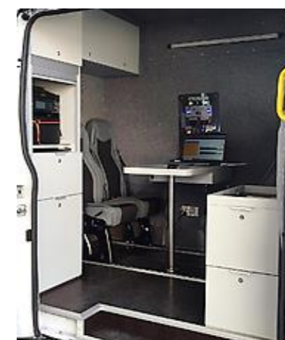
Operators' compartment consisting of MDS control panel for switching monitors, cameras, charging, etc., a laptop with RPM software, a wall-mounted alarming module and multiple supplementary equipment
