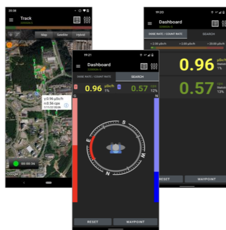
Polismart® iOS and Android app for wireless BRD operation allowing to monitor the measurements in real time, record the GPS-referenced waypoints, export and transfer the records
