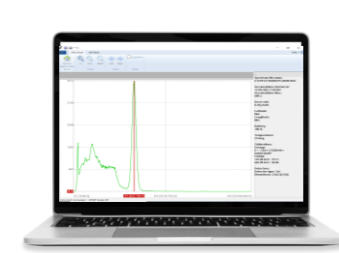
User Software for adjusting settings, downloading the operating history and analyzing the gamma spectra
