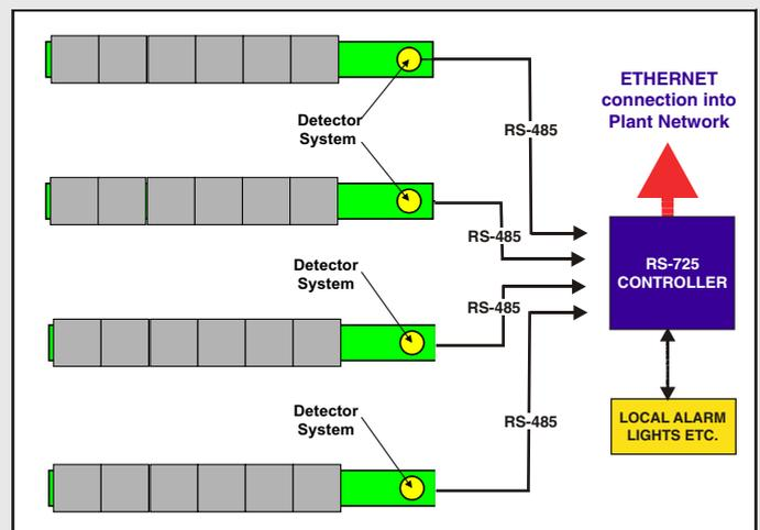
*The RS-725 Controller is connected directly to the Plant Network via the Ethernet port giving the RSO direct access to alarm data.*
