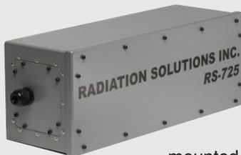
The **RS-725/21** system is a 3"x3" (21 cu ins) Sodium-Iodide detector mounted in a square housing. Normally the face of the detector is
