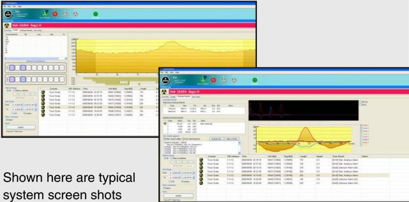
Shown here are typical system screen shots which illustrate what a total count alarm looks like as well as the spectral analysis of this alarm. In addition, Internet connection to the RSI Service Center gives the RSO outside technical support capability for problem alarms.
