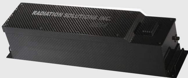
The **RS-725/128** system is a 4 x 2 x 16" (128 cu in) Sodium-Iodide detector with internal 0.5" lead shielding to reduce background and "focus" the detector. Mounting of the detector is recommended to be located 4-6" from the monitoring point depending on local conditions. Since the detector is internally collimated only a basic mounting structure is required to position the detector where required.
